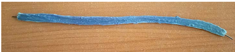
Fig. 5. A 150 mm nitinol wire is coated with a sky-blue microencapsulated thermochromic pigment achieved by impregnating liquid latex rubber with a sky-blue thermochromic pigment. The coating texture is coarse and uneven due to the use of the paintbrush method to coat the wire's surface.
