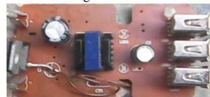
Fig. 7. The Front view of the internal circuitry of the customized DC charger
