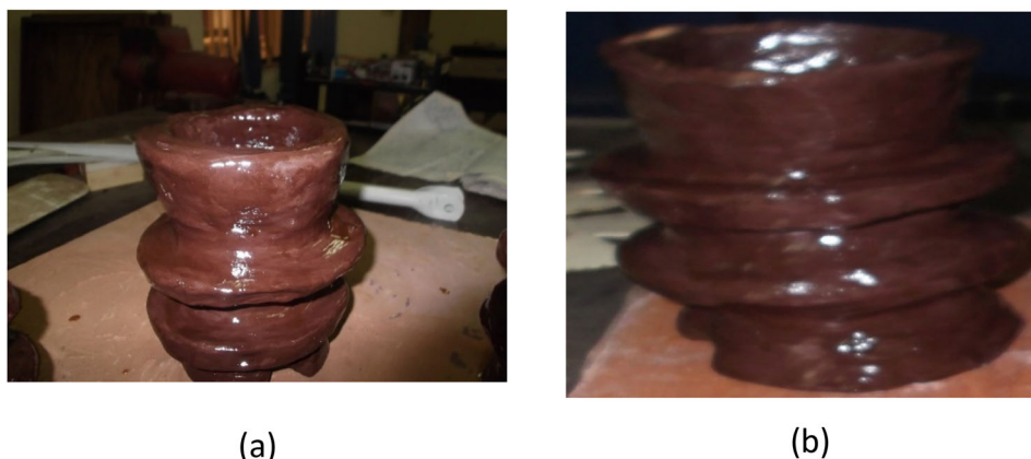
Figure 4. Sample of the clay insulator after. (a) Applying the glaze. (b) The application of gloss.
