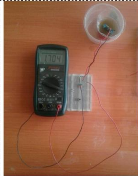
Figure 2b. Caustic potash solution (KOH) is used as electrolyte for air battery and produces a voltage of 1.704V
