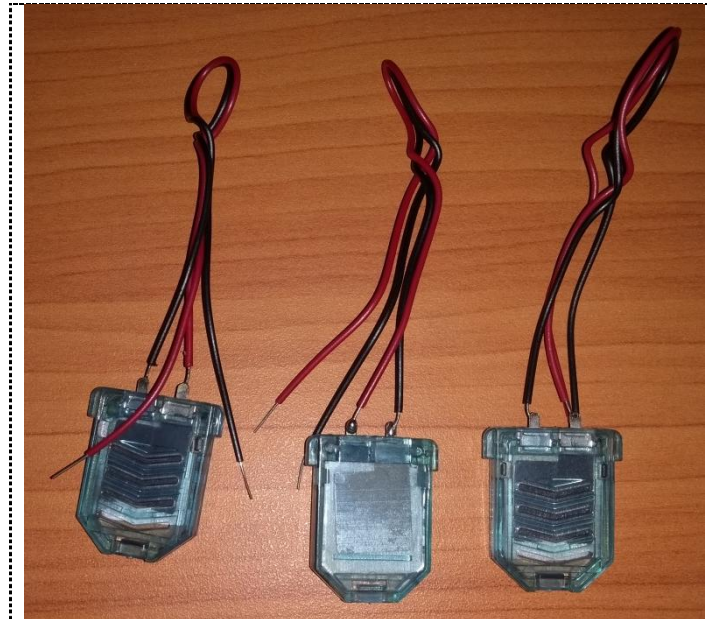
Figure 1. Three metal-air electrodes that make use of aluminium metal as anode material
