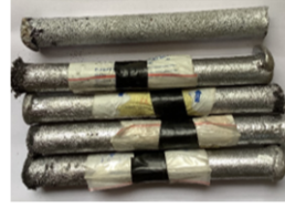
Figure 2. Reinforced Aluminium Matrix Composite.
