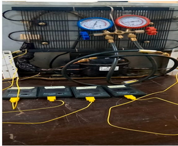
Fig. 2. Experimental set up of the refrigeration system.
