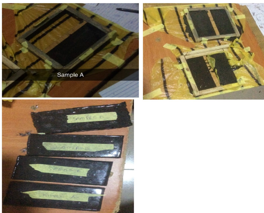
Fig. 8 Pouring of the mixture into mould boxes and produced samples
