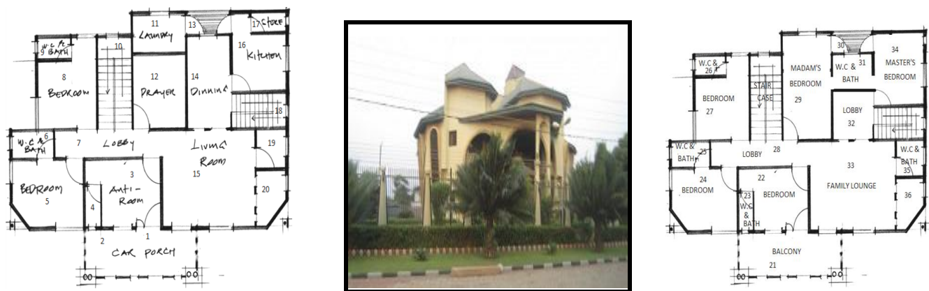
Figure 12: Ground, Upper Floor Plan and Picture of a Detached Double Floor Villa House Source: Ekhaese, (2011)
