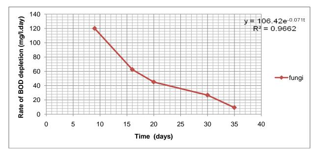
Fig 7: Effect of Fungi (Aspergillus Niger) on the Rate of Depletion of BOD of Treated Crude Oil Polluted Water with Time
