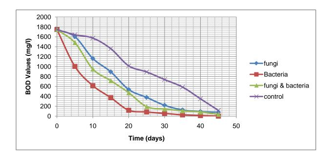
Fig.2: BOD Values for Aerobic Bioremediation of Treated Crude Oil Polluted Water
