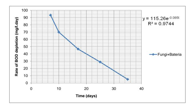
Fig.6 Effect of Combined Bacteria and Fungi on the Rate of Depletion of BOD of Treated Crude Oil Polluted Water with Time
