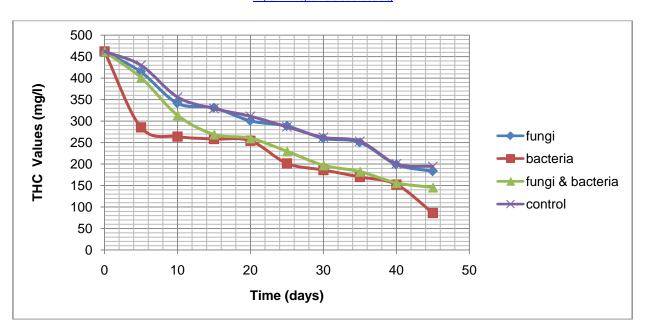
Fig.3: THC Values for Aerobic Bioremediation of Raw Crude Oil Polluted Water
