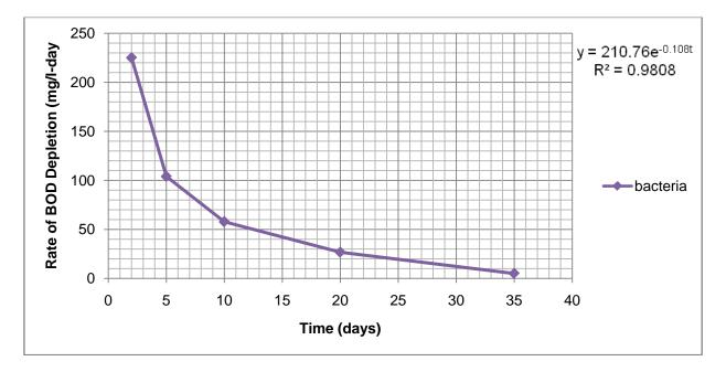
Fig.5 Effect of Bacteria on the Rate of Depletion of BOD of Treated Crude Oil Polluted Water with Time
