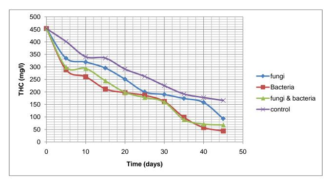
Fig.4: THC Values for Aerobic Bioremediation of Treated Crude Oil Polluted Water
