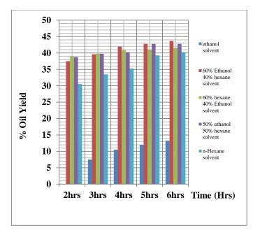
Figure 2: Oil Yield obtained during Neem Oil Extraction at different Time using Ethanol, Hexane and their combinations
