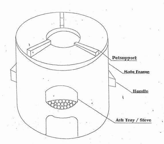
Fig. 1: Am Isometric View of Fire Clay Stove
