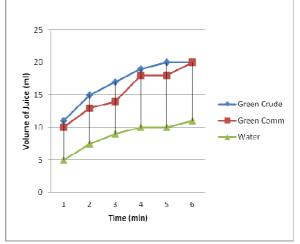
**Fig 7:** Clarification of Green apple juice with 30ml crude pectinase, commercially produced pectinase and water
