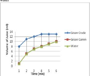
**Fig 4:** Clarification of Green apple juice with 20ml crude pectinase, commercially produced pectinase and water
