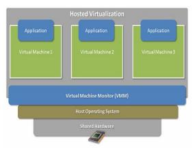
Figure 1. Hosted virtualization architecture, virtual machine monitor (VMM) software is installed on a host operating system [18].
