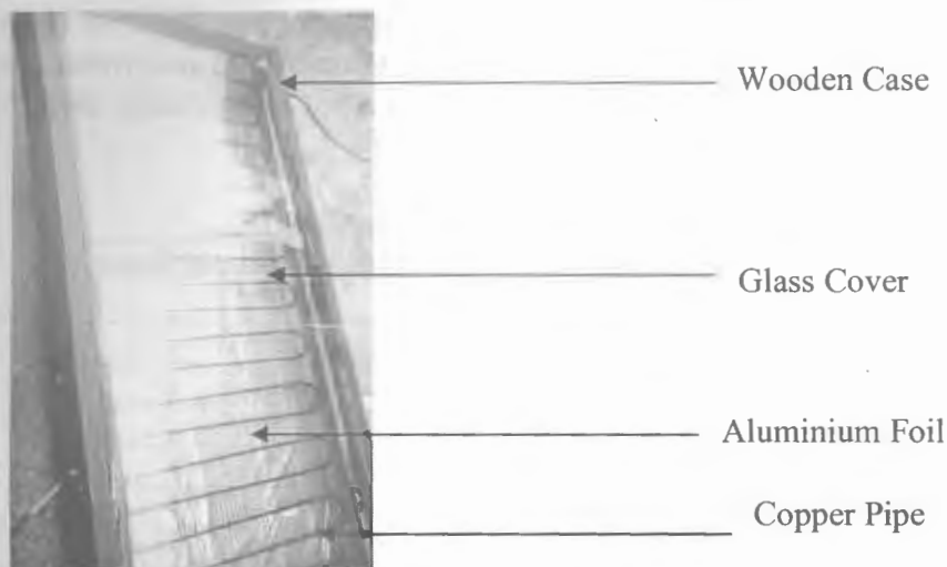
Figure 1: Solar water heating ( heat collector) system
