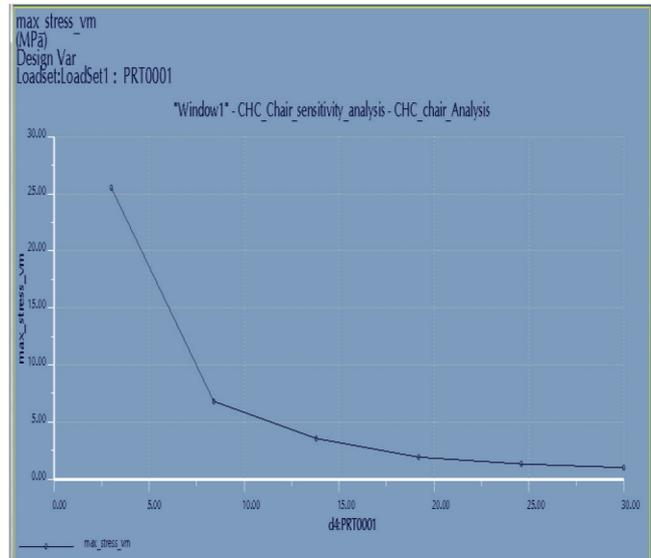
Fig 2: Stress (Mpa) against the thickness of the cattle horn – plastic composite chair seat.
