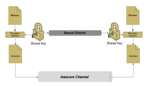
FIGURE .2.1 : Simplified model of conventional encryption (Mohammed *et al.*, 2011)
