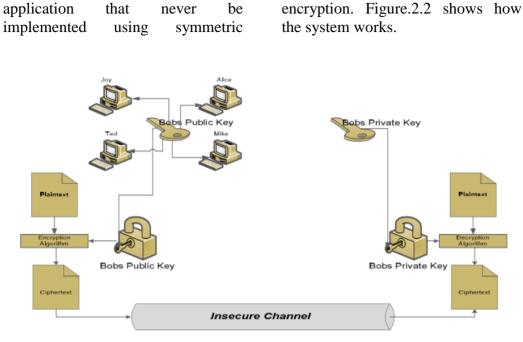
FIGURE 2.2 : Simplified model of asymmetric encryption (Mohammed *et al.,* 2011)
