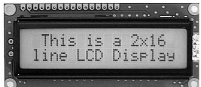
Figure 9: A 16 by 2 LCD module
