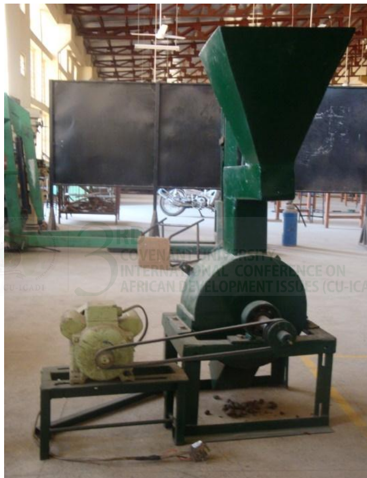
Fig. 4: A pictorial view of the palm kernel cracking machine
