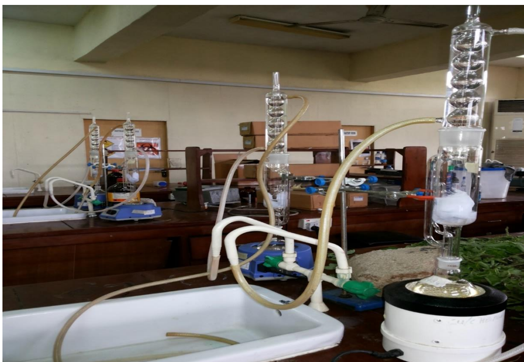
Figure 3.7 A set up of Soxhlet apparatus for the extraction of crude fat
