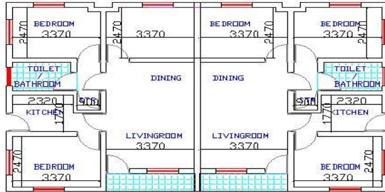
Figure 5.4: Original 3-bedroom semi-detached bungalow in Federal Low Income Housing Estates program, Australia, 2009
