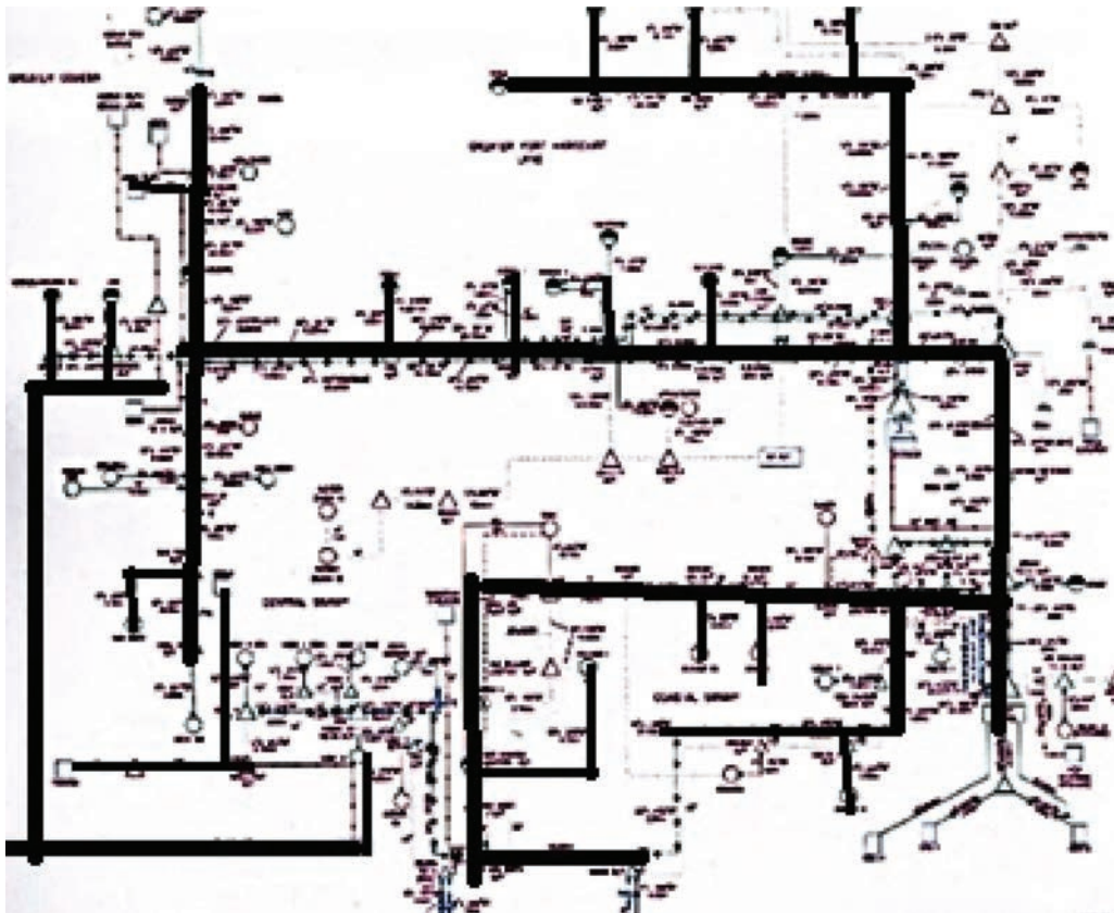
Fig. 3—Typical crude-oil-pipeline network.
