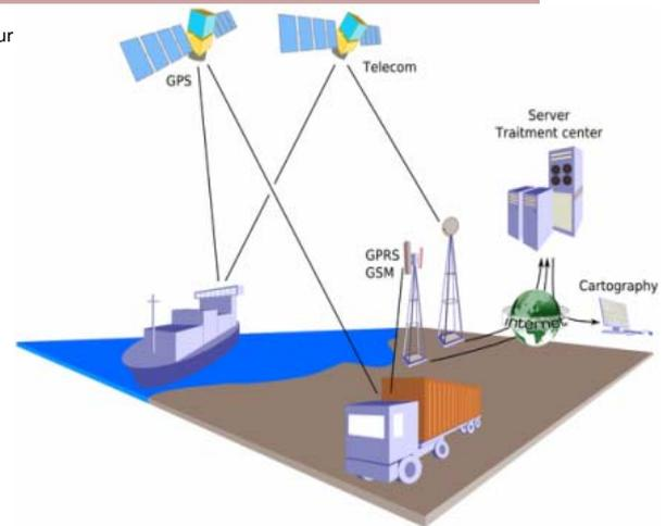
**Fig. 2:** Application of Satcom for tracking
