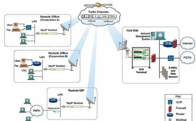
Fig. 1: Satellite Communication deployment scenario for Internet Access
