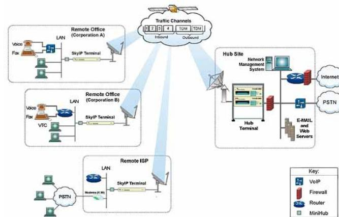
**Fig. 1:** Satellite Communication deployment scenario for Internet Access
