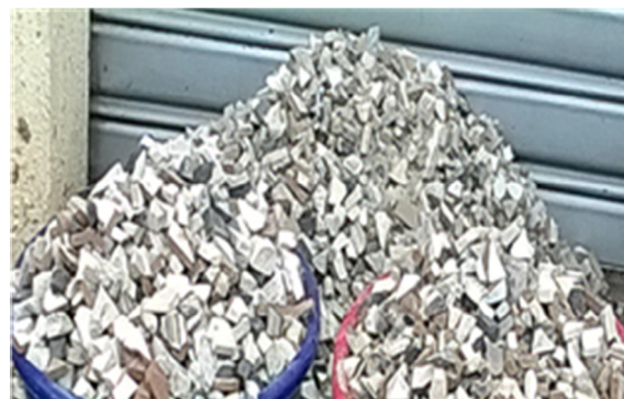
Fig. 1b Ceramic aggregates after crushing and grading.
