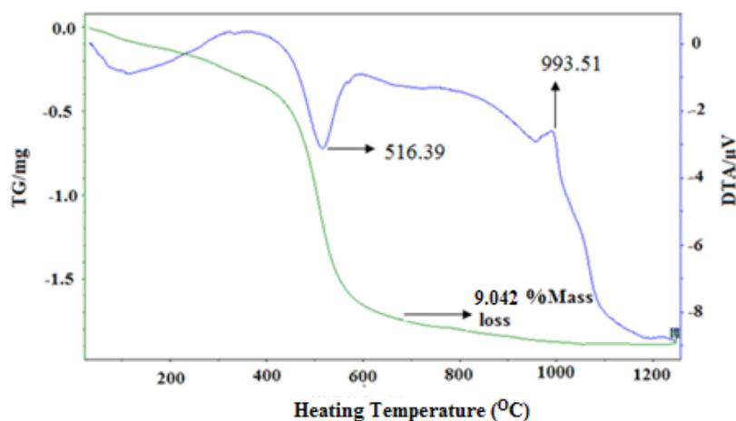
Fig. 1: Simultaneous thermo gravimetric and differential thermal analysis of processed clay
