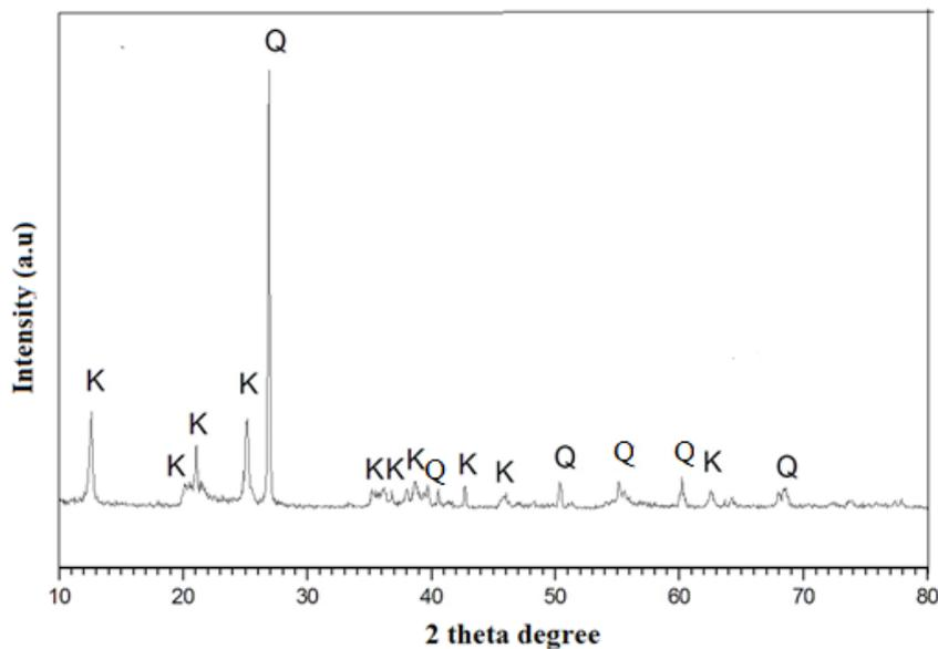
Fig. 3: X-Ray Diffraction pattern of processed Clay sample [K=Kaolinite, Q=Quartz]
