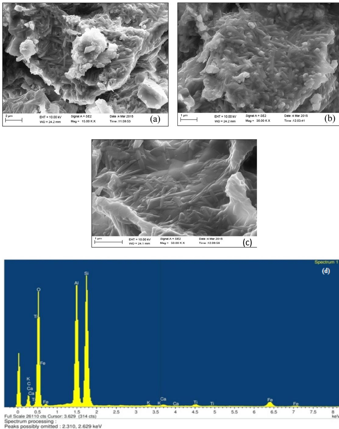
Fig. 7: Photomicrograph at 1400°C at different position and magnification
