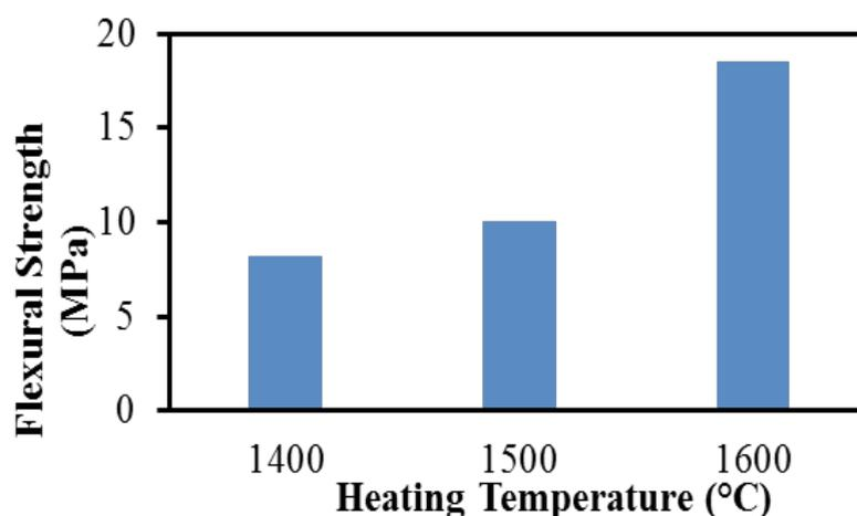
Fig. 5: Variation in flexural strength of fired clay samples with heating temperature
