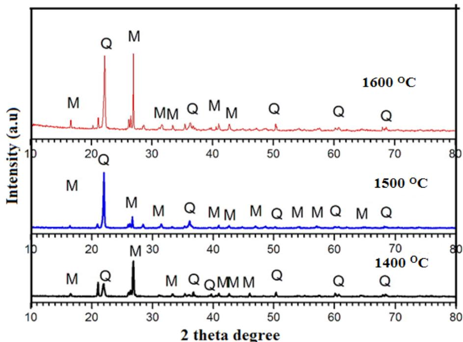
Fig. 6: XRD pattern of the fired Clay samples
