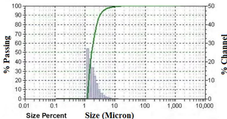
Fig. 2: Particle size analysis of processed clay powder
