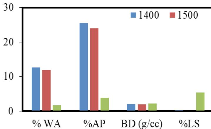
Fig. 4: Variation in LS, BD, WA and AP of fired Clay samples with heating temperature
