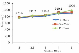
Figure 9: Steady increase in latency as file sizes increases
