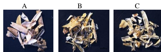
Figure 4: Stereoscope micrographs taken at 1000 μm scale of the untreated (A), Pretreated (B), and enzymatic digested (C) rice husks
