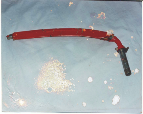
Figure 2: Failed Landing gear
