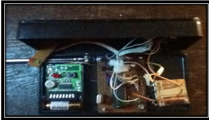
Figure 7. Remote Control (Transmitter Unit)
