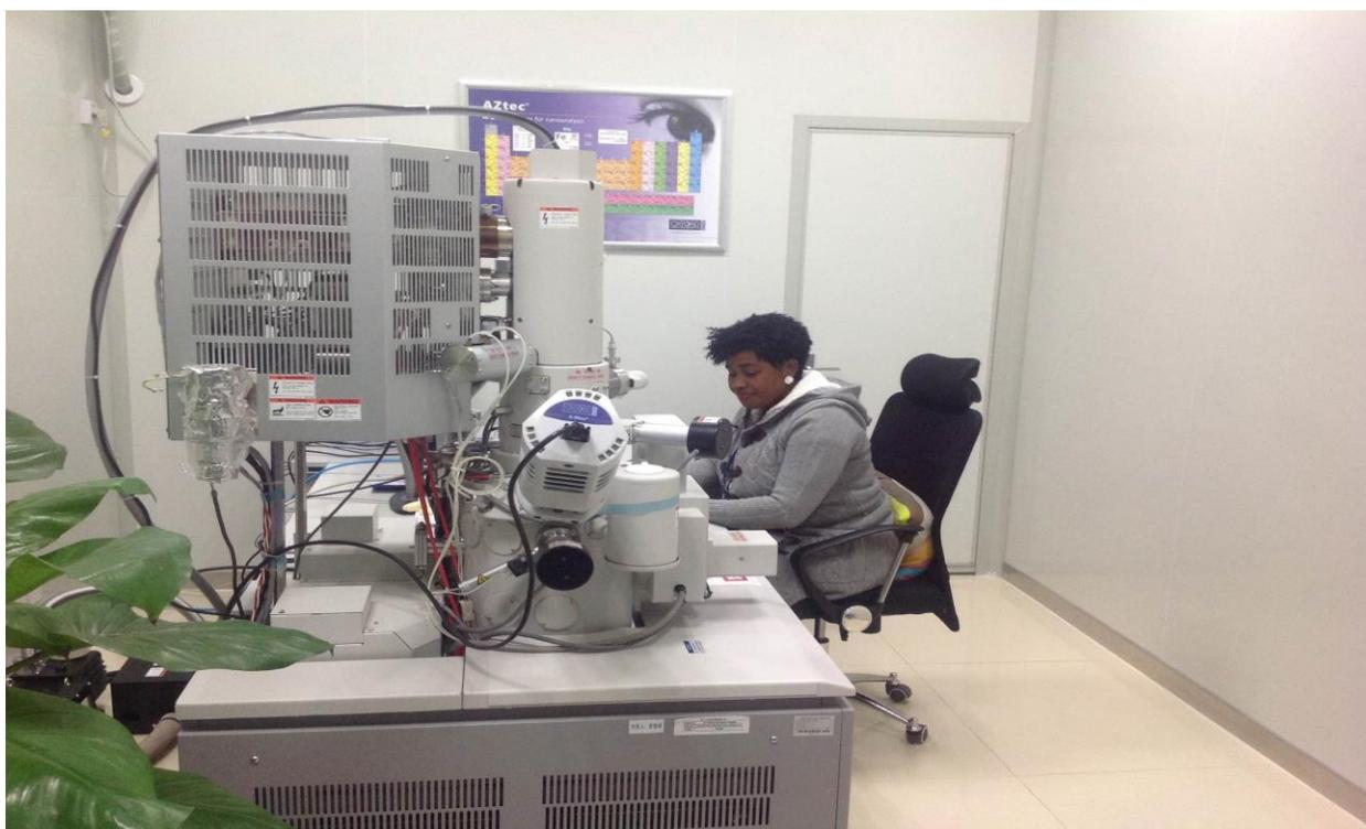
Plate 4: Morphology analysis of PM<sub>2.5</sub> filters using Field emission scanning electron microscopy- energy-dispersive X-ray spectroscopy (Hitachi, SU-8020).
