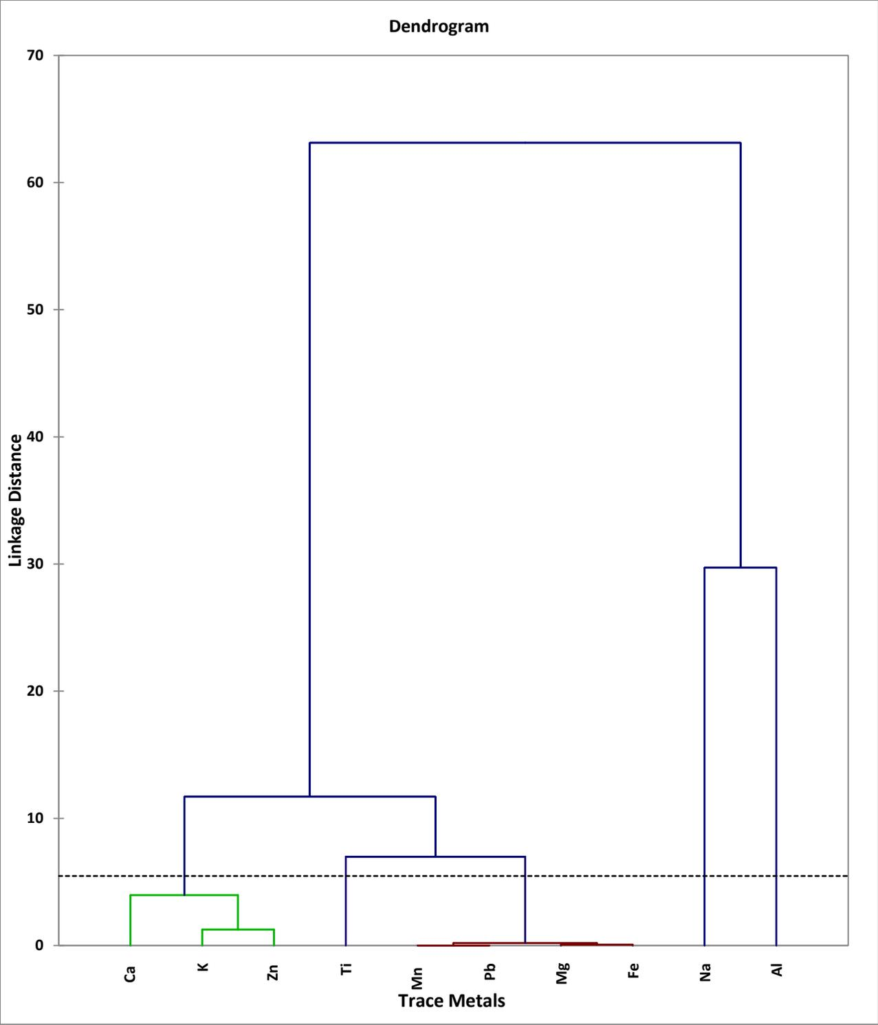
Figure 4.21: Dendrogram showing different trace metals clusters in AGE
