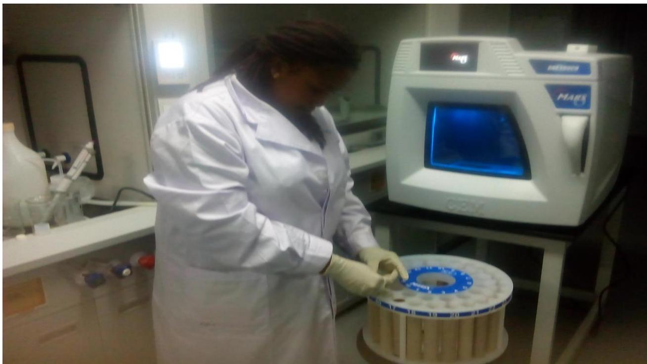
Plate 6: Sequential extraction analysis using CEM MARS 6 microwave reaction system
