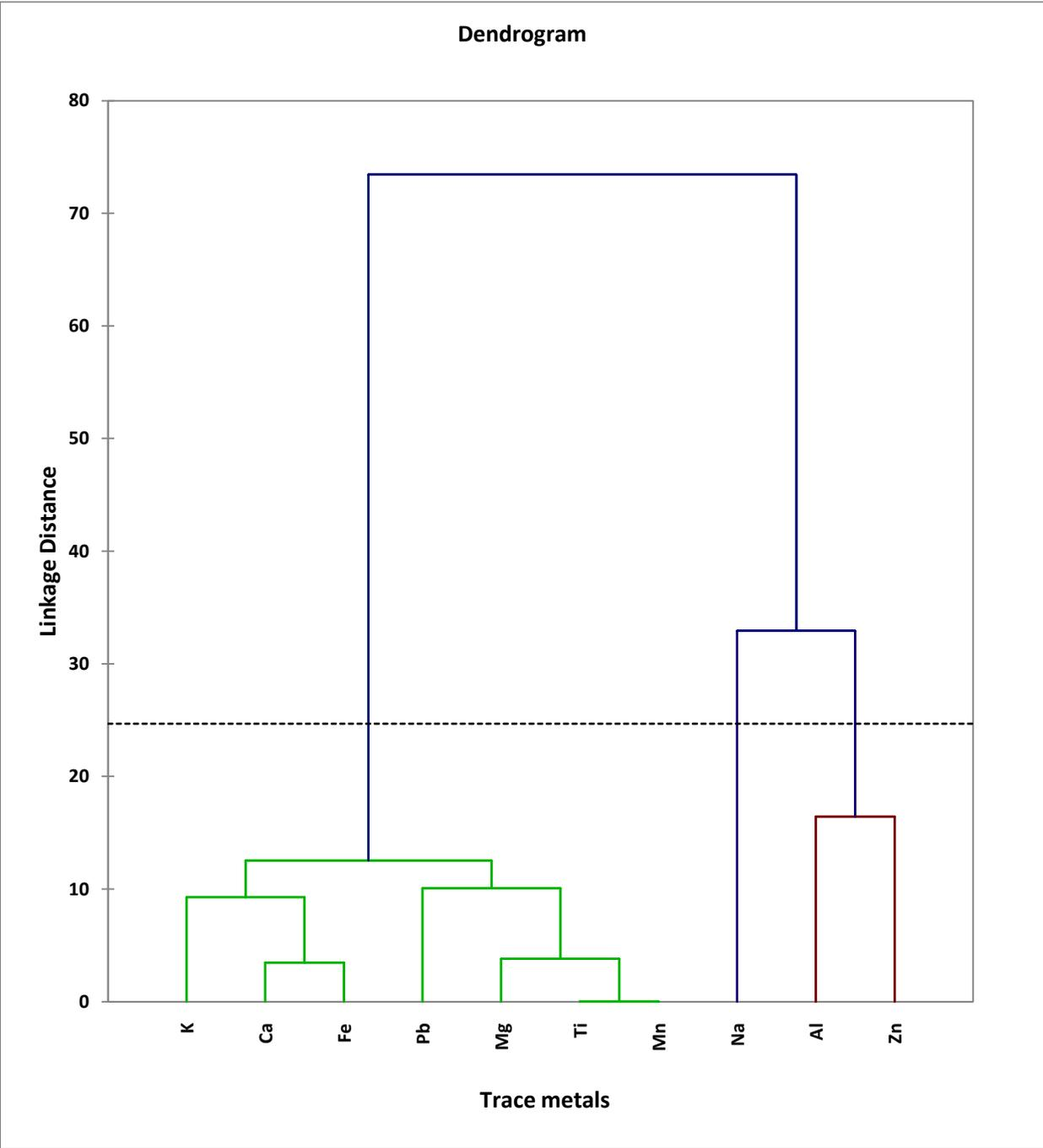
Figure 4.20: Dendrogram showing different trace metals clusters in OTE
