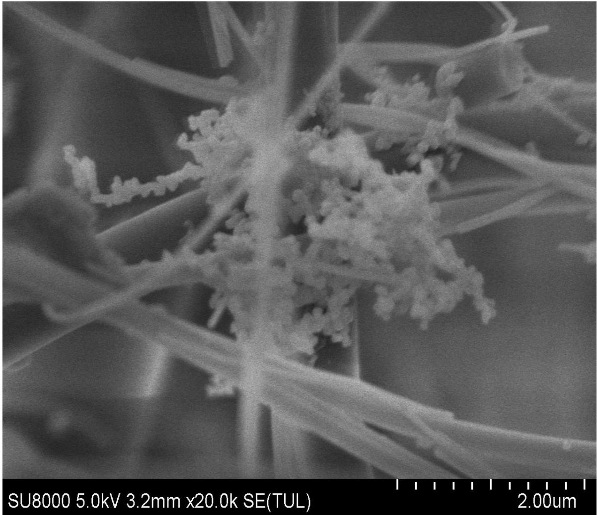
**Figure 4.12: Morphology of PM<sub>2.5</sub> soot particles at EWC during the dry season**
