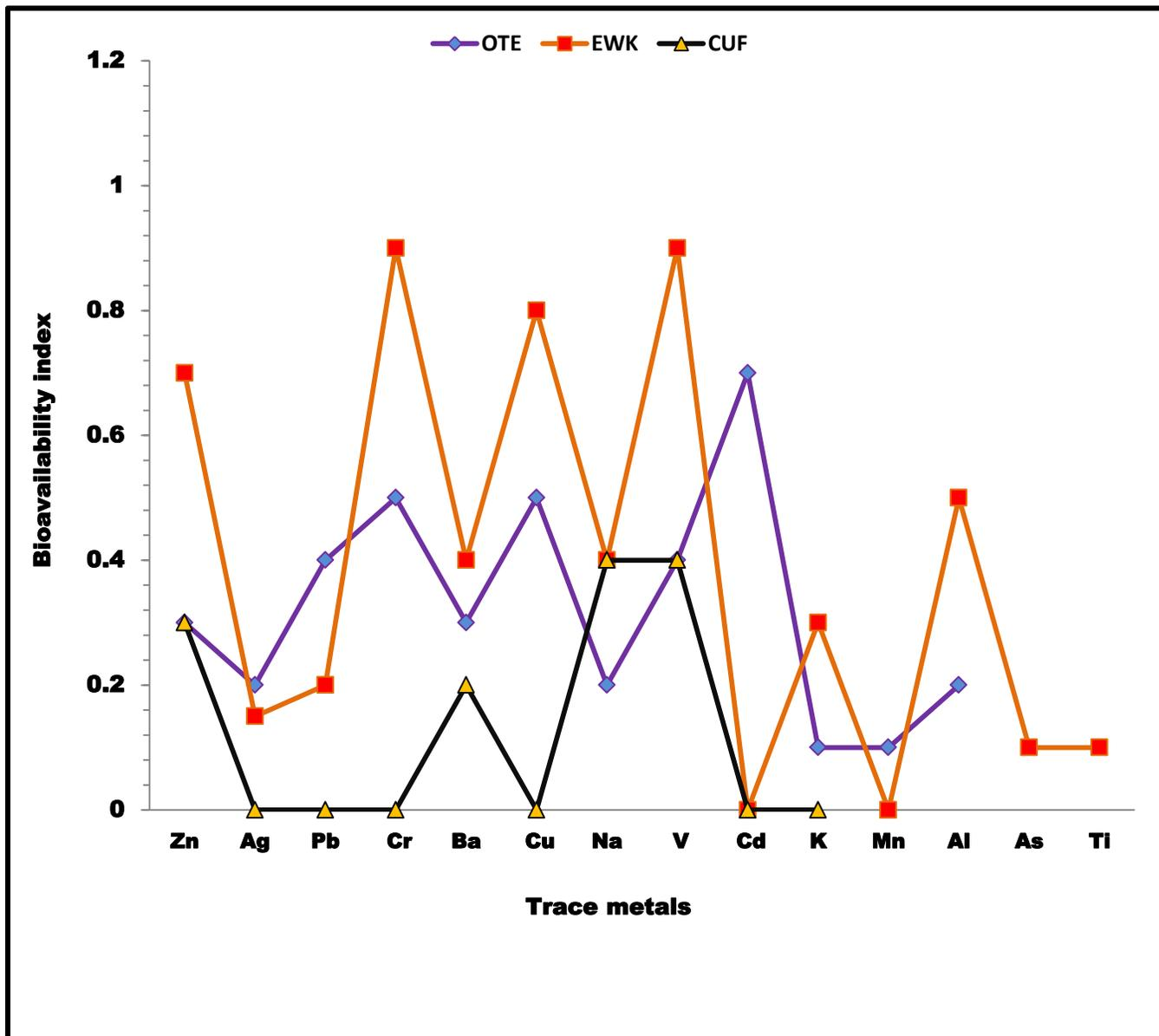
Figure 4.6: Bioavailability index of PM<sub>2.5</sub>-bound trace metals
