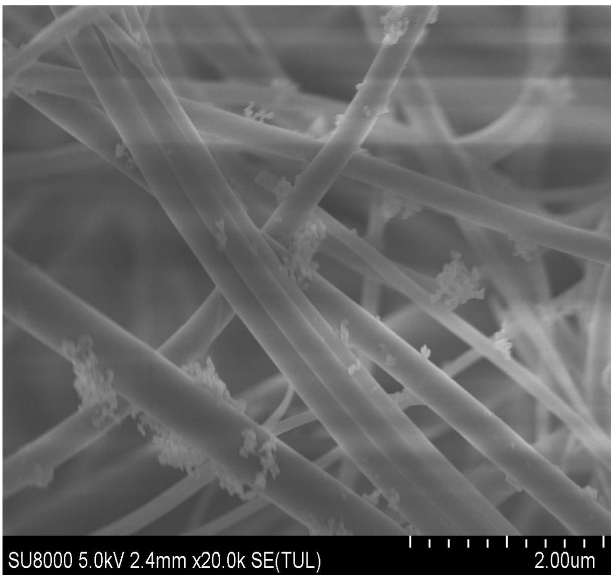
**Figure 4.13: Morphology of PM<sub>2.5</sub> soot particles at AGE during the dry season**
