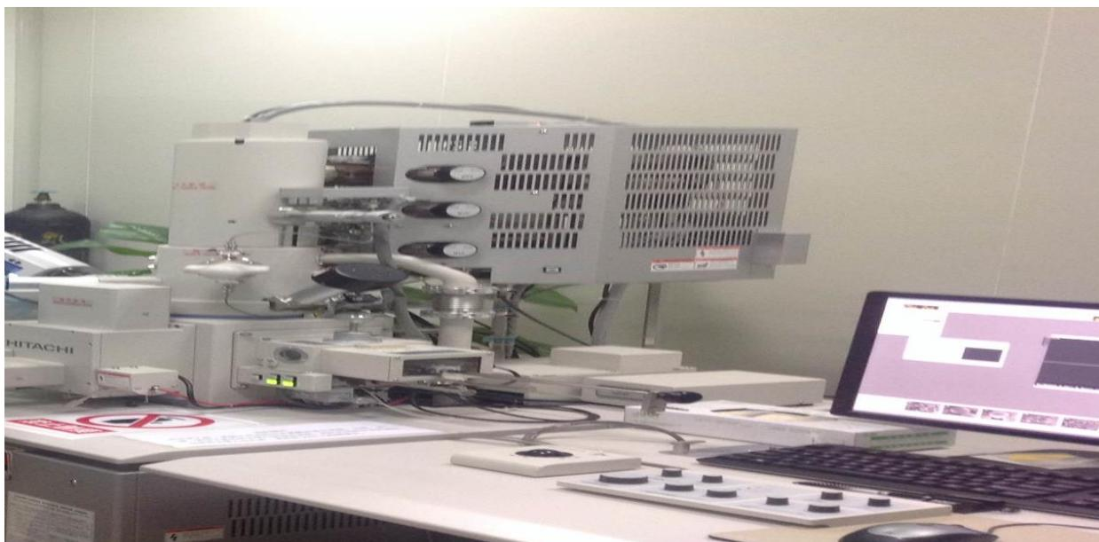
Plate 3: Field emission scanning electron microscopy- energy-dispersive X-ray spectroscopy (Hitachi, SU-8020).
