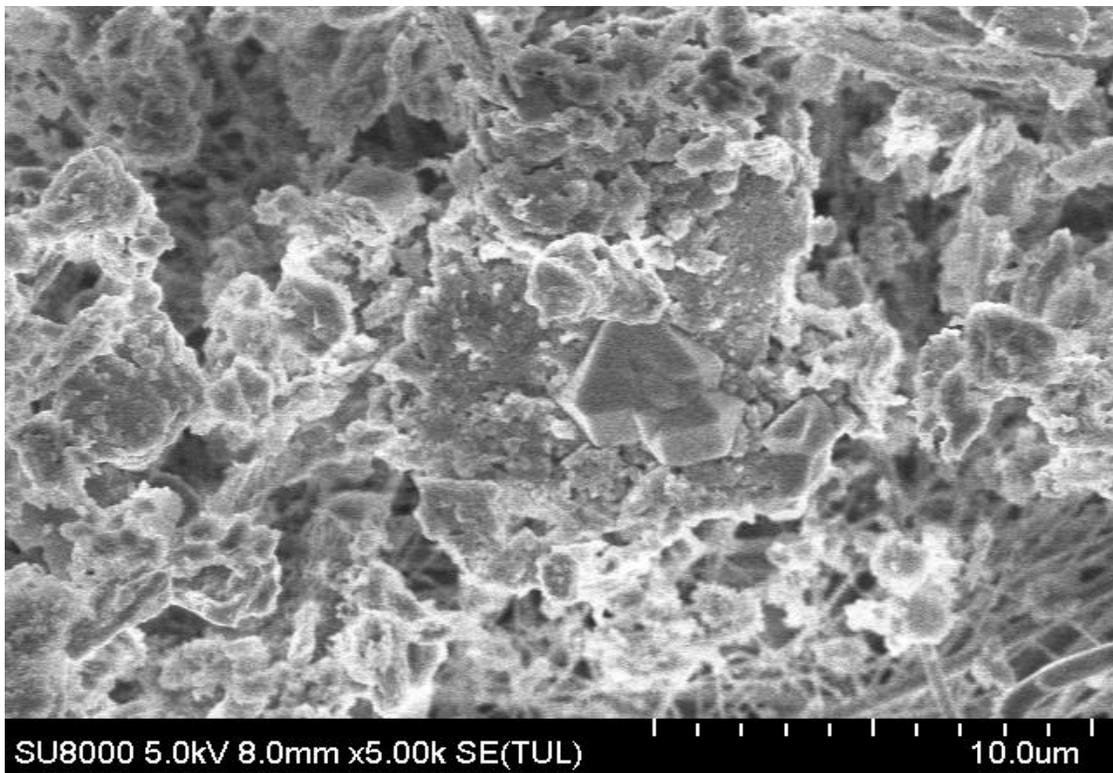
Figure 4.15b: Morphology of PM<sub>2.5</sub> fly ash particles at EWC during the dry season
