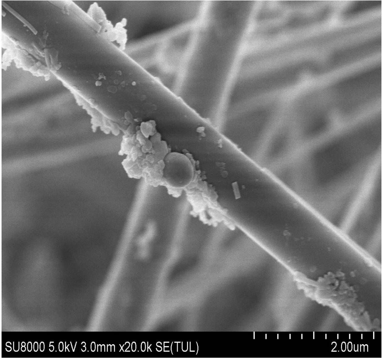
**Figure 4.14: Morphology of PM<sub>2.5</sub> soot particles at OTE during the wet season**
