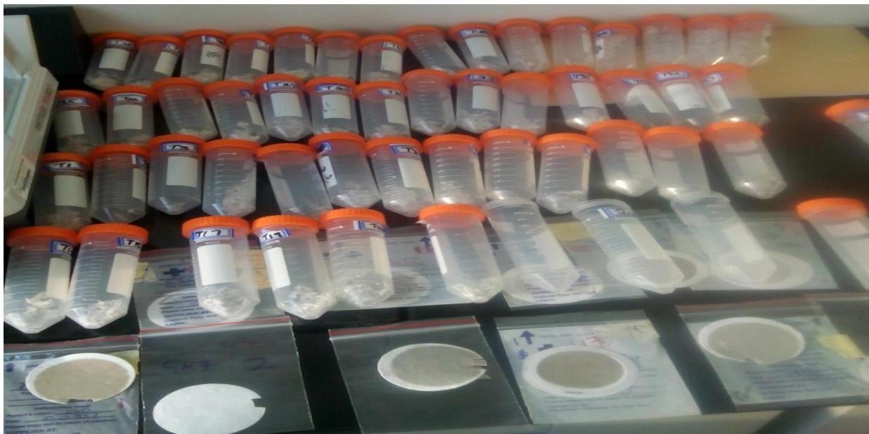
Plate 5: Samples of filters for trace metals analysis
