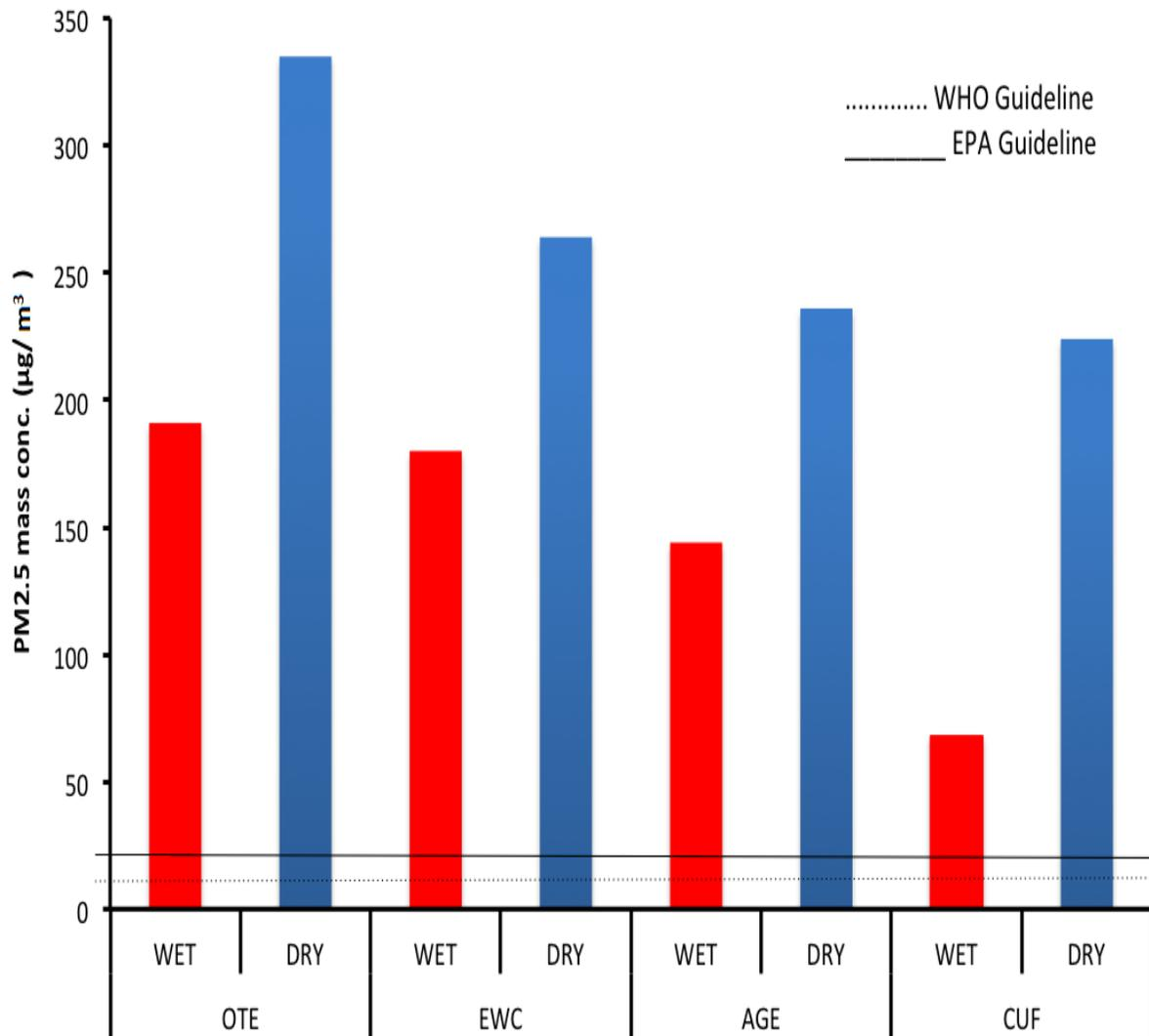
**Figure 4.1: Average seasonal concentration of airborne PM<sub>2.5</sub> in all the study areas. Horizontal lines indicate the 24-h standard limits established by US-EPA and WHO**
