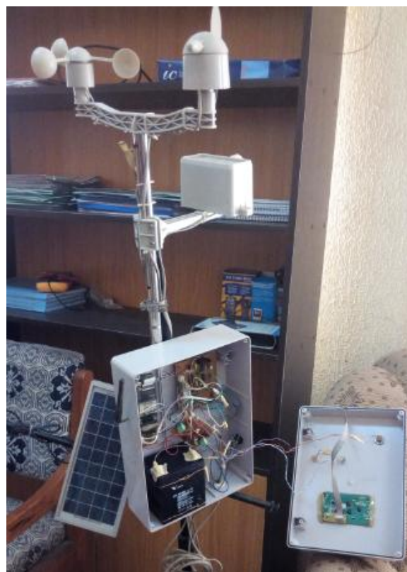
Figure 3: Automated Weather Station
