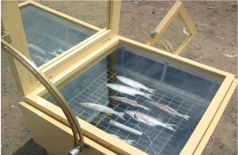
Solar Cabinet Fish Dryer.
