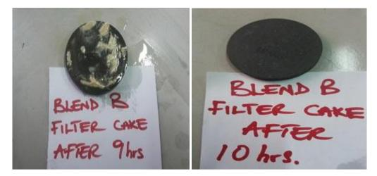
There was a complete clean-up after **10hrs** in the soak solution \* We had a total break through time of 2hrs 45mins
