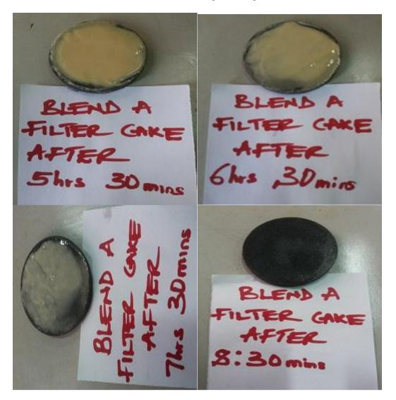
There was a complete clean-up after **8hrs 30mins** in the soak solution. \*We had a total break through time of 2hrs.
