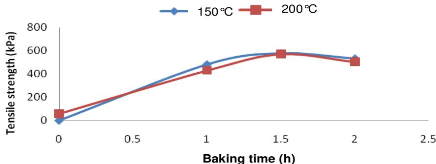
**Figure 7.** Plot showing the effect of increasing temperature on the strength of core with Palm oil strength at constant baking time.
