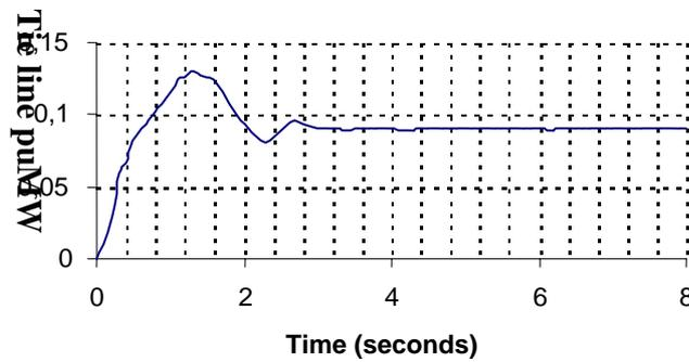
Fig. 5 Tie-line power transient.
