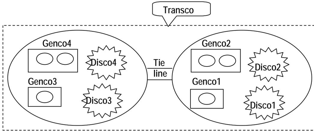
**Fig.1 Two area control structure**
