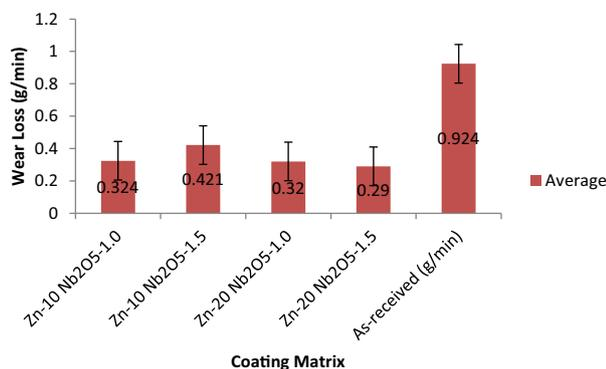
Fig. 7 Wear plastic deformation trend of fabricated Zn-Nb<sub>2</sub>O<sub>5</sub> on mild steel
