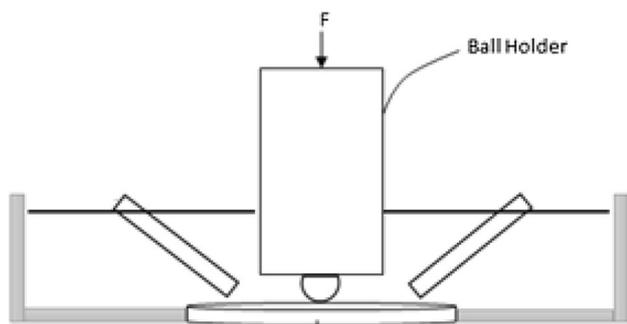
**Fig. 1** Schematic view of reciprocating sliding friction CERT UMT-2 test system
