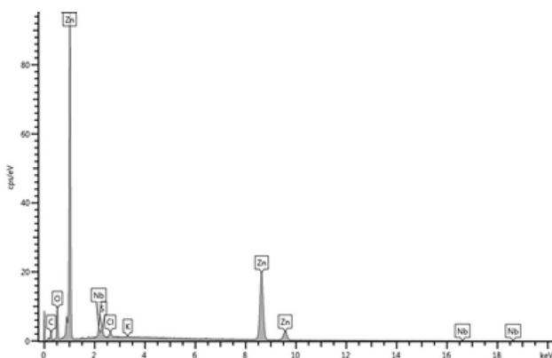
**Fig. 3** EDS pattern of fabricated Zn– $\text{Nb}_2\text{O}_5$ -20 g at  $1.5 \text{ A/dm}^2$
