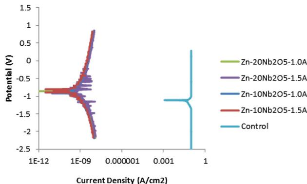
Fig. 8 Potentiodynamic polarization curves of Zn-Nb<sub>2</sub>O<sub>5</sub> composite coating on mild steel in 3.65% NaCl solution
