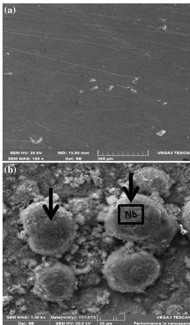
**Fig. 2** SEM spectra of **a** as-received mild steel **b** Zn–Nb<sub>2</sub>O<sub>5</sub>-20 g at 1.5 A/dm<sup>2</sup>
