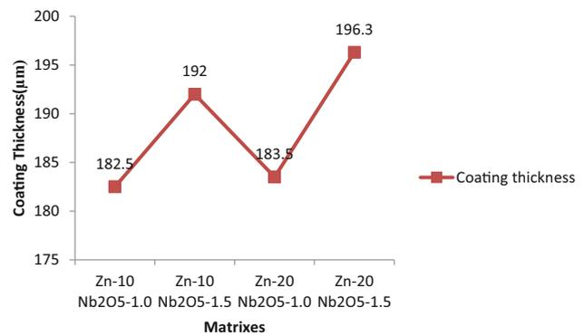
**Fig. 4** Coating thickness progression of fabricated Zn– $\text{Nb}_2\text{O}_5$  on mild steel
