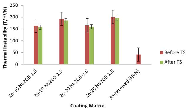
Fig. 6 Thermal stability of fabricated Zn-Nb<sub>2</sub>O<sub>5</sub> on mild steel
