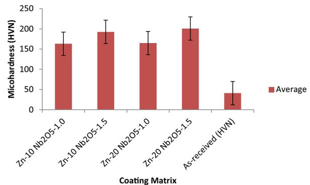
**Fig. 5** Microhardness progression of fabricated Zn– $\text{Nb}_2\text{O}_5$  on mild steel before heat treatment
