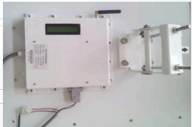
Figure 2. Re-engineered UHF Antenna with LCD Interface & Wireless Antenna
