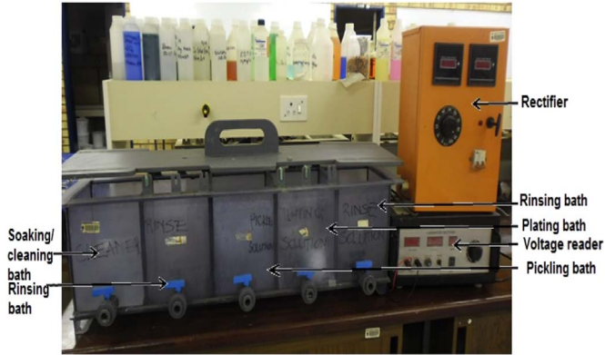
Fig. 1. Electroplating setup.
