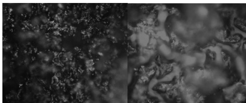
Figure 13. Optical micrograph images of mild steel after corrosion with HPD inhibitor from HCl solution (a) mag.x40, (b) mag.x100
