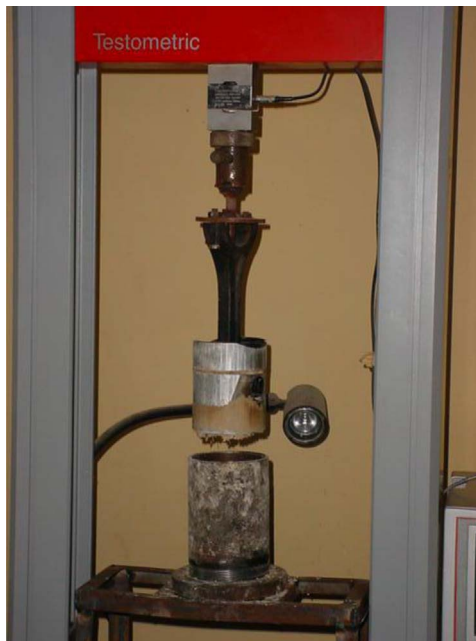
Fig. 6. Showing the Piston-Cylinder Assembly on the Universal Testing Machine.
