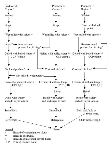
Fig. 1. Preparation of kunun-zaki by producers A–C. \*, Hazard of contamination likely; \*\*, hazards of survival; +, hazards of microbial growth likely; CCP, critical control point.
